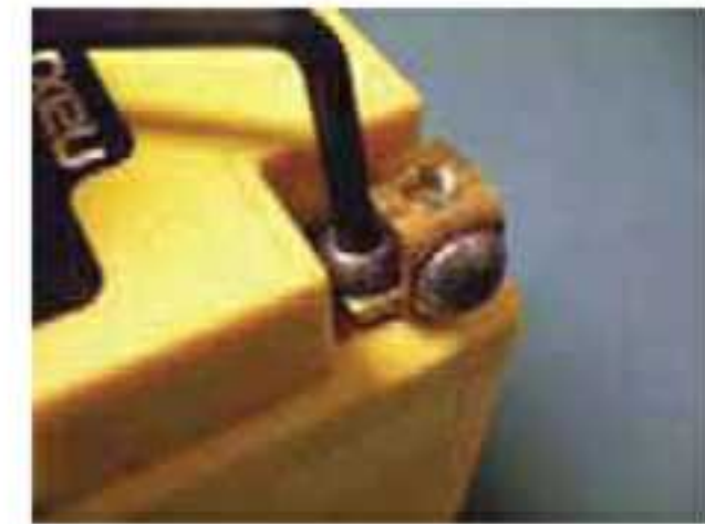
Attaching the terminals
