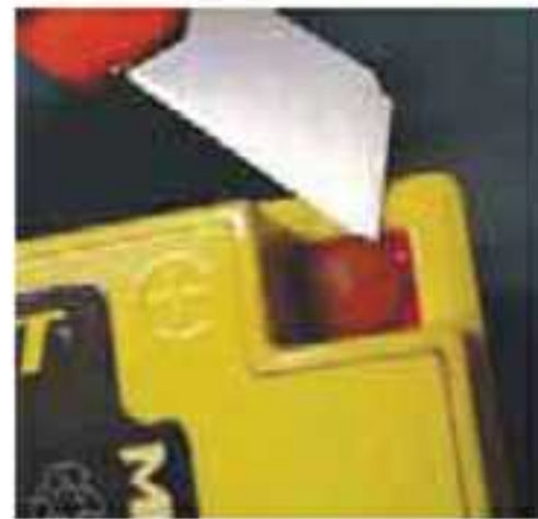
Removal of terminal plugs
